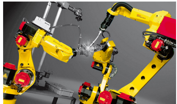
Fig. 1: Laser welding performed by three cooperative Robot.
