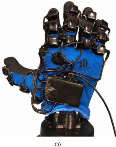
Fig. 2. Figure a) shows the SoftGlove worn by a Pisa/IIT SoftHand, with some circuitry details, before the waterproofing. Figure b) shows its waterproof version, mounted on the waterproof SoftHand.
