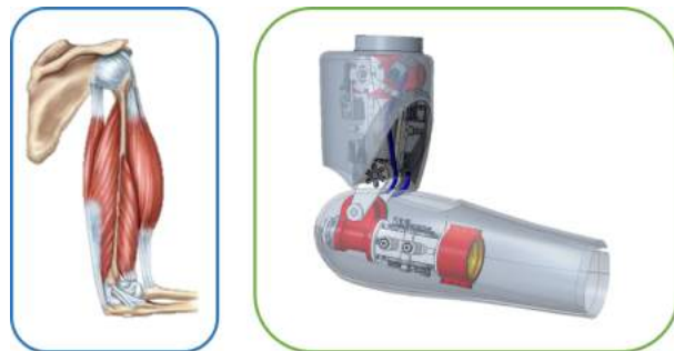
Fig. 1. Each human joint is activated by at least two muscles. Human beings control their impedance through posture and co-contraction. The picture shows the musculoskeletal scheme of the elbow joint (left) and the mechanical implementation (right) of the articulated soft elbow prosthetic joint presented in this work.
