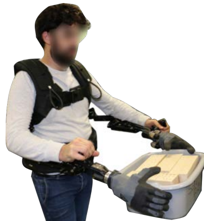
Fig. 1: In picture, a user using the supernumerary robotic arm-hand system for holding a box. Main parts of the system are the gravity compensatory arms (Armor Man 2.0, Tilta) and the soft robotic hand (Pisa/IIT SoftHand [6]), connected by a customized damping wrist.
