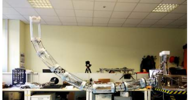
Fig. 1. Prototype of the inspection robot assembled with 5 modules
