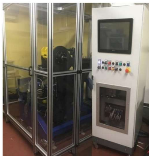
Fig. 5. Test bench for PHM on EMA flight controls [2]
