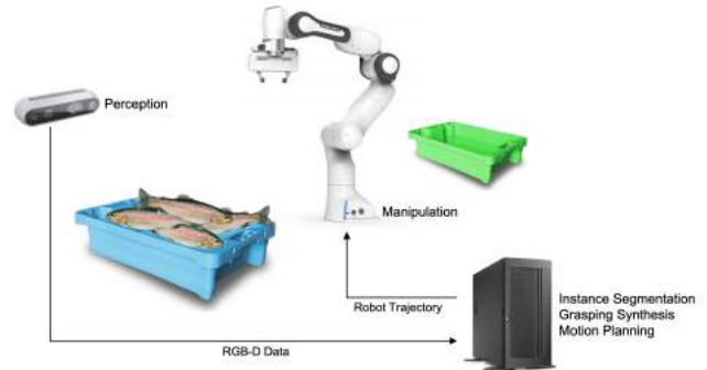
Fig. 1: SPIWI project concept: a robot accurately transfers fresh fish from large bins to small trays, ensuring with a predictive weighing procedure that the total weight of each tray is kept within specified limits.
