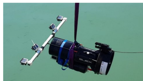
Figure 1 - SDS employed during the mission, acoustic transponder below the scooter, cameras on the left [2]
