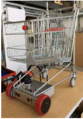
Fig. 3. Robotized shopping trolley used for the BEAST benchmark. The box houses motors, electronics and communication gear.
