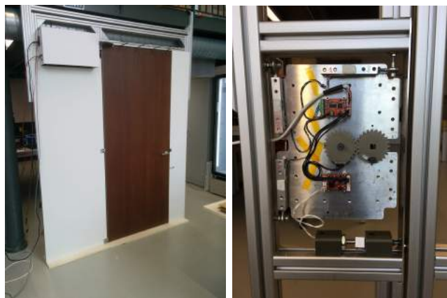
Fig. 1. Robotized door used for MADROB benchmark. The fully assembled door (left) and a detail of the lock assembly (right) internal structure.
