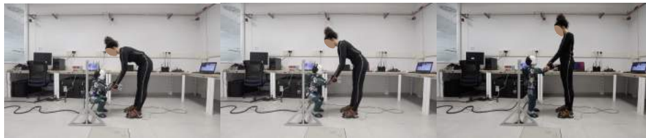
Fig. 1: Experimental scenario with the iCub humanoid robot standing-up with the help of a sensorized human.
