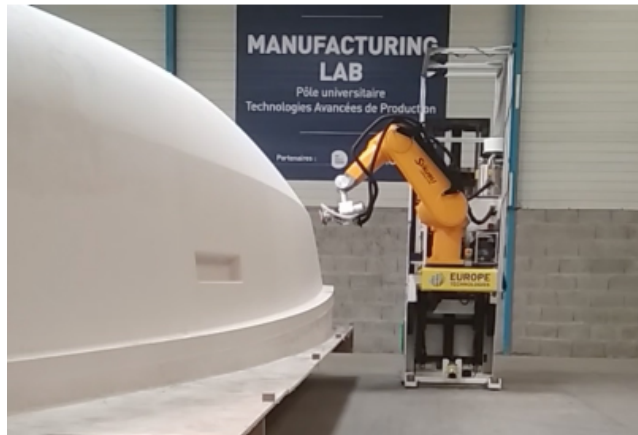
Fig. 1: Example of the industrial scenario considered in the COROMA project, including a boat hull and the sanding robot.
