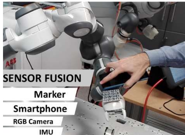
Fig. 1. The method enables the user to jog the robot in contactless way by using a common smartphone.
