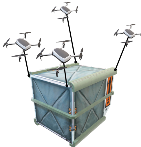
Fig. 1. A cable-suspended object manipulated by multiple aerial robots.
