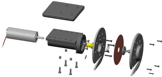
Fig. 2. Exploded view of the cutting end-effector. The cutter is attached to the robot via a flange. The actuation is composed of an electric motor with a planetary gearbox. The circular blade, with a diameter of 60 mm and a thickness of 0.6 mm, is protected by a frame.
