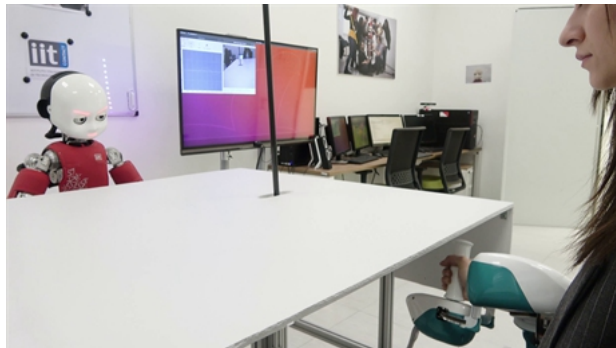
Fig. 1: The robot looking at the pendulum with a focused expression while the participant tries to balance it by using the Wristbot.
