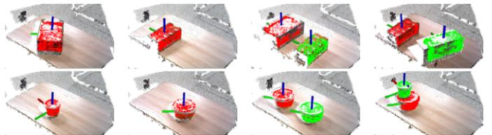
Fig. 4. The output of the perception algorithm is shown overlaid on the point cloud of the scene.
