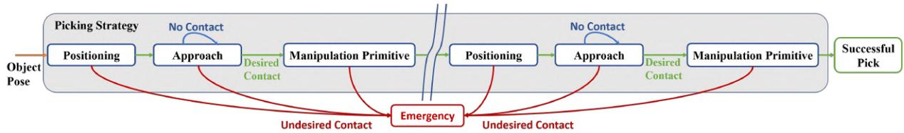
Fig. 2. General Scheme of the Reactive Planning Framework
