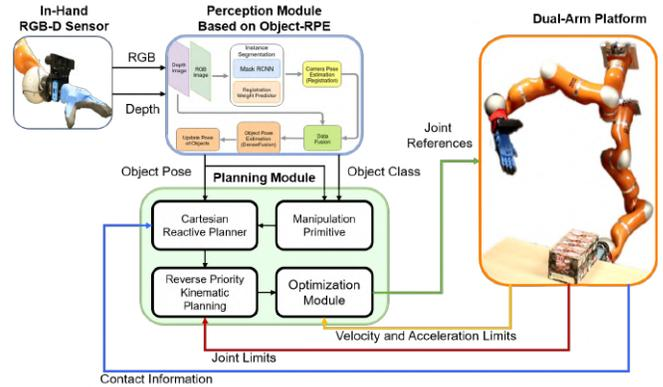
Fig. 1. Block scheme of the integrated system. The reactive planner algorithm, that take as input the information given by the perception system, is used to adapt and re-plan online the picking strategy based on contact information from force torque sensors at the end-effectors.
